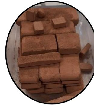
Briquetted sewage sludge ash
